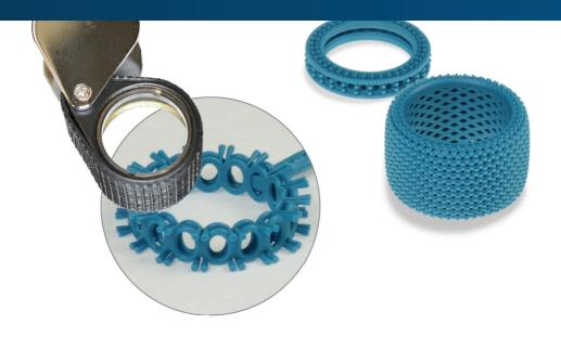
With Solidscape, we do not worry about adding support wires to our designs. The system factors in where support is needed for us, saving time in both CAD and at the bench during finishing."
